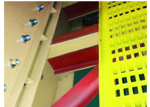
Screen deck frames can be lined with Linatex® premium rubber products as an additional option
